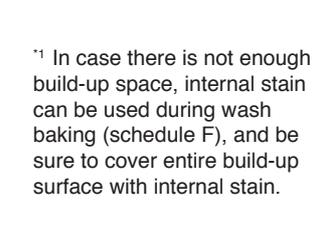
\*1 In case there is not enough build-up space, internal stain can be used during wash baking (schedule F), and be sure to cover entire build-up surface with internal stain.
